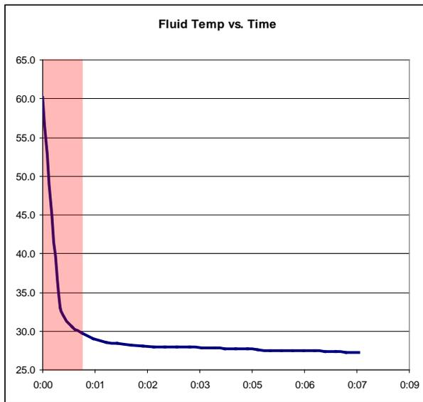
The rate of change (time vs. temperature) is very steep, and there is not time for the fluid, instrument, and ambient temperature to come to an equilibrium. Although the instrument has automatic temperature compensation, the rate of change is so steep that it is impossible to get a stable reading for nearly the first 60 seconds.
